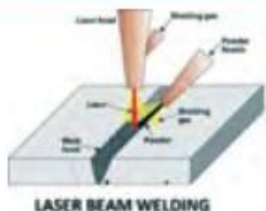
Laser beam welding (LBW) 레이저빔 용접 Hàn tia laze
