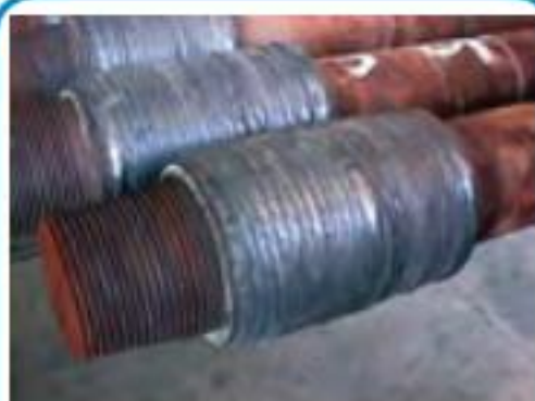
Built-up welding 덧붙이 용접 Hàn bổ sung
