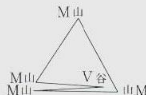
図2: 凸立体角折りの切り口 / Figure 2: The cross-section of a convex solid angle fold.
